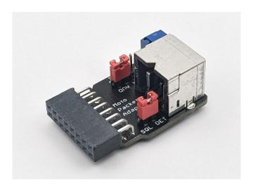
This adapter makes connecting a packet TNC, APRS Tracker or any other 1200/9600 baud data modem to a Motorola mobile radio with the standard rear panel 16 pin accessory port easy!
