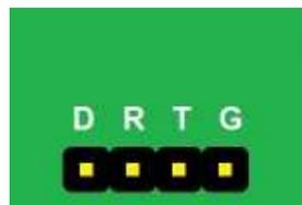
**Important:** When the RTrak-HAB is not being programmed, the included jumper block must be in place over the first two pins marked “D” and “R”, in order for the GPS data to be passed to the OpenTracker 1+!
